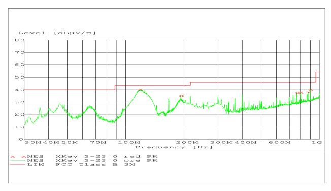
Plot 3 - Radiated Emissions - 30MHz to 1GHz
