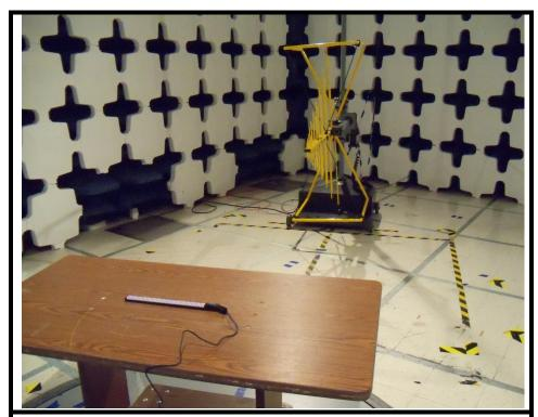
Test Setup Photo 2 – Radiated Emissions
